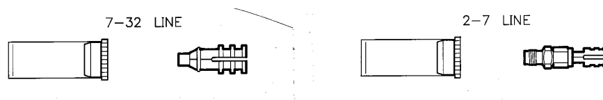
Figure 1-2 Line Standards — 7 to 32 GHz and 2 to 7 GHz Air Lines Installed in Tools with Storage Bottles
