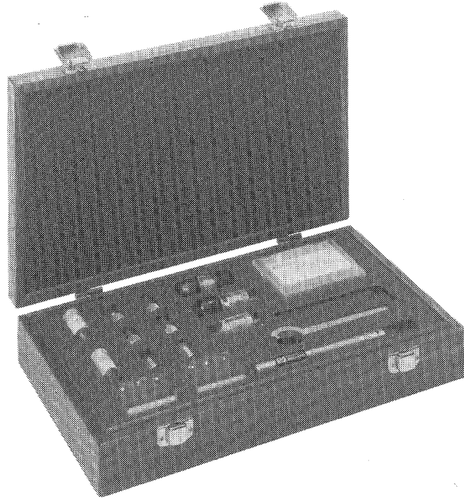
Figure 1-1 85052C Precision Calibration Kit
